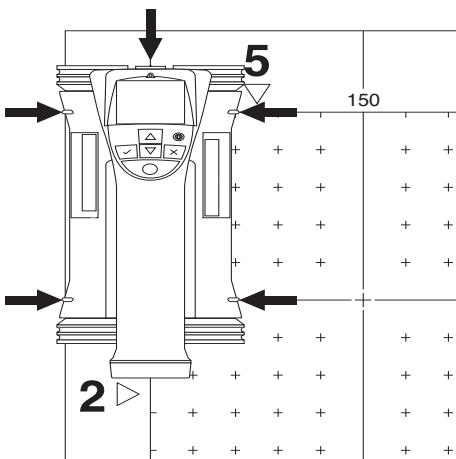
Place the scanner on the grid at the starting point shown by the blinking arrow. Ensure the alignment marks on the scanner are aligned correctly with the reference grid as shown above.
