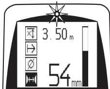
The bar is positioned along the center line of the scanner and may be marked on the surface using a PUA 70 marking pen. Depth measurement accuracy can be increased by entering the correct rebar diameter or by switching to accurate depth measurement measuring mode (see 7.2.5.2).
