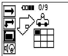
Switch the scanner on and use the Arrow buttons to select the Blockscan symbol from the main menu. The battery level is displayed together with the number of Imagescans currently held in memory (a maximum of 9).
