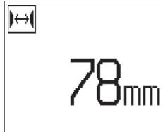
If the spacing distance is known, the value can also be entered manually using the Arrow buttons.
