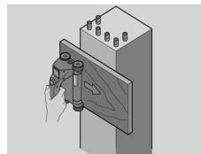
Use a thin sheet of non-metallic material (e.g. cardboard, wood, polystyrene foam,...) as an overlay that extends beyond the edge. The scanner can then be moved over the sheet to beyond the edge of the structure. Note that the thickness of the board must be deducted from any depth measurements. The thickness of the board can be entered in the PC application. This value will then be automatically deducted from any depth measurements.
