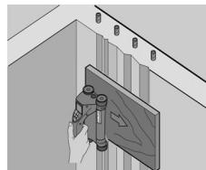
Rough surfaces (e.g. concrete surfaces with exposed aggregates) cause additional noise in the signal and may mean that the depth or diameter of a bar cannot be determined. In such cases it is also advantageous to scan through a thin overlay board. Also in this case, the thickness of the board must be deducted from any depth measurements.
