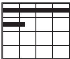
Press Record and move the scanner along the first row. Scanning progress is indicated by a thick black line that advances across the display as the scanner is moved over the surface.
