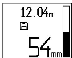
To record the position and depth of all reinforcing bars detected, place the scanner on the surface and use Quickscan detection to find a position where there are no bars present. Mark the starting point with a PUA 70 marking pen and press the Record button. The diskette symbol appears on the screen, indicating that the scanner is recording data. Move the scanner over the surface.
