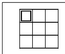
A representation of a Blockscan is shown on the screen. Each square represents an Imagescan. Up to 3 x 3 Imagescans can be made. Use the Arrow buttons to select the position of the first Imagescan to be made. Press Confirm to begin the first Imagescan. Note that the coordinates of any points on the Blockscan will be referenced from the upper left corner.
