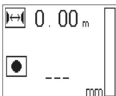
The bar spacing distance can be calculated automatically using the Quickscan detection function by searching for the center of the bar and pressing the red Record button when the scanner is over the mid point of the bar. Find the mid point of the next bar and then press the Record button again. Bar spacing is then calculated automatically and recorded.
