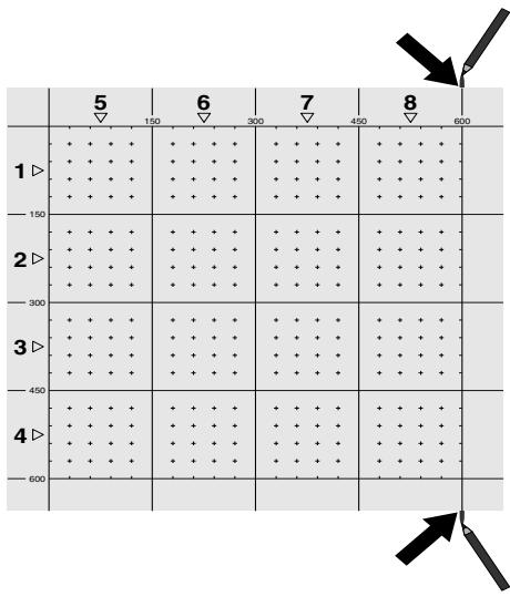
Attach the reference grid in the same way as for an Imagescan. Use a PUA 70 marking pen to mark the edges or the punched holes at the end of each reference grid for the transition to the next grid, as shown below. Any additional reference grids required should be attached to the wall so that their edges correspond and are in alignment with each other.
