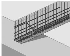
In cases where the reinforcement must not be damaged, ensure that Imagescans are made on at least three sides
