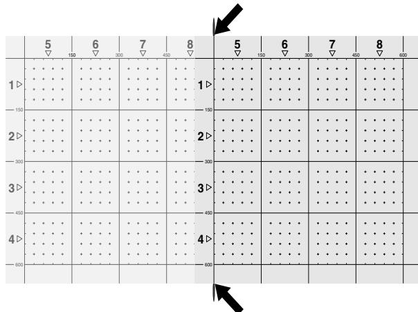
Select the next Imagescan position and repeat the scanning procedure. Imagescans already made may be repeated simply by reselecting the area to scan and carrying out the Imagescan again. The data will be overwritten. Once all the Imagescans have been recorded, or the maximum number of scans that can be held in memory is reached (9), press the Cancel button to return to the main menu. Transfer the data to the monitor for viewing and analysis (see 7.4.1).
