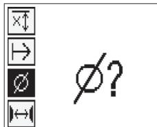
If no bar diameter is selected, the scanner will take the average diameter value for the relevant standard setting range and calculate the depth accordingly.
