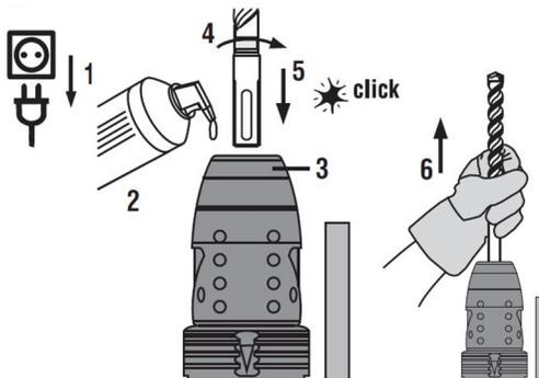
1. Apply a little grease to the connection end of the accessory tool.
