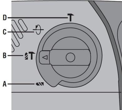
1. Set the function selector switch to the **T** position.
