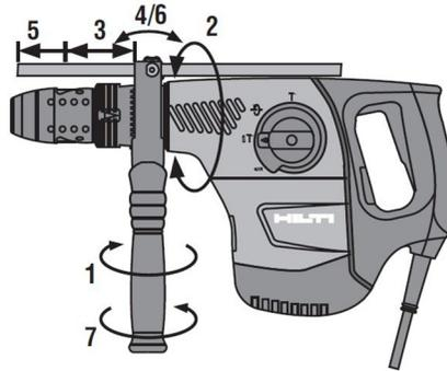
1. Release the side handle clamping band by turning the handle grip.
