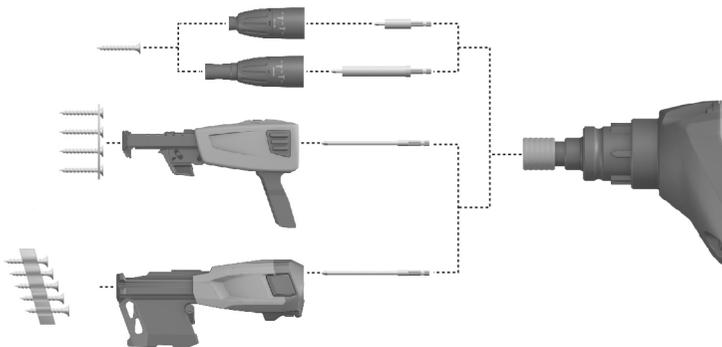
1. Pull the depth gauge away from the power tool, releasing the snap-on connection.
