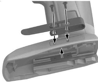
The belt hook enables you to attach suitable power tools to your belt. It can be fitted to allow attachment on the left or right side of the body.
