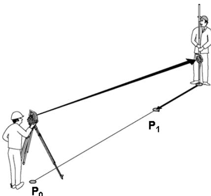
**P<sub>0</sub>** is the position of the tool after setting up.
