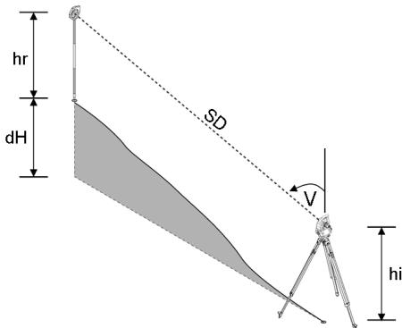
The height measurements take the **vertical angle** and the **slope distance** in conjunction with the **instrument height** and the **reflector height** into account.
