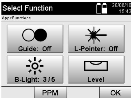
Switch the laser pointer on/off.
