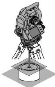
Lay a piece of paper, plastic foil or other semi-translucent material on the pipe in order to make the laser point visible.
