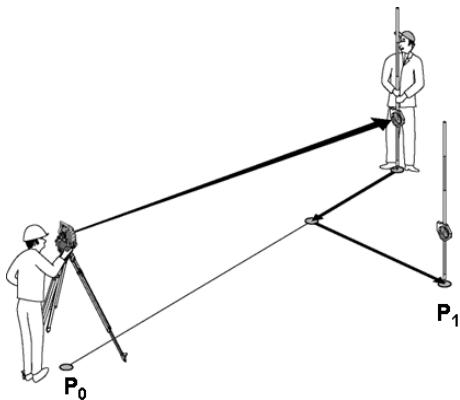
**P<sub>0</sub>** is the position of the tool after setting up.
