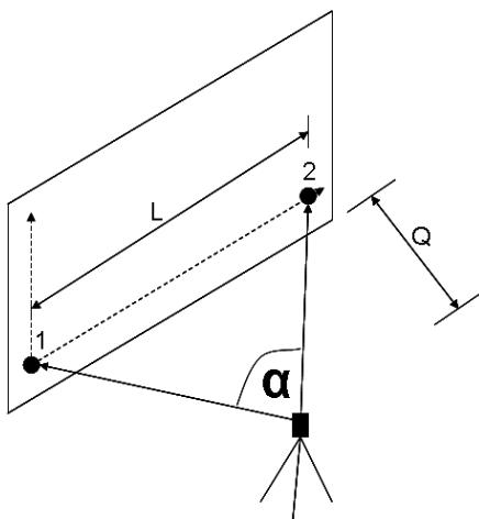
An optimum setup or, respectively, tool position has been achieved when the ratio between the horizontal reference length  $L$  and the distance  $Q$  is  $L : Q = 25 : 10$  to  $7 : 10$ , so that the included angle lies between  $\alpha = 40^\circ - 100^\circ$ .
