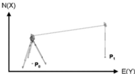
The tool is positioned at a point defined by coordinates **P0** and, for the purpose of orientation, is aimed at another point defined by coordinates **P1**.
