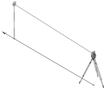
The laser beam takes measurements to "normal" surfaces without need for a special reflector.
