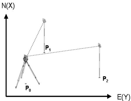
The tool is positioned at any desired point **P0** and is then used to measure, one after the other, the angle and distance to two reference points with known coordinates **P1** and **P2**.
