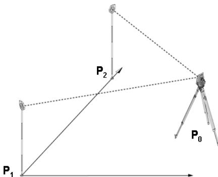
The position of the tool **P0** is not on the building control line. The measurement to the first reference point **P1** fixes the beginning of the control line, while the second measurement **P2** records the direction of the building control line in the system.
