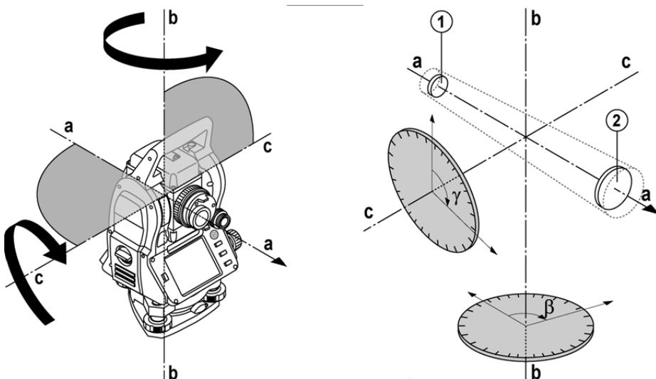
Tool inclination is determined with the aid of electronic levels (compensators), circle readings are corrected accordingly and the height difference is also calculated from the measured slope distance and horizontal distance.
