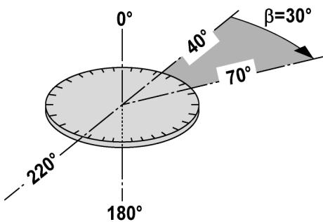
The included angle of  $70^\circ - 40^\circ = 30^\circ$  can be calculated from the horizontal circle readings of  $70^\circ$  to one target and  $30^\circ$  to the other target.
