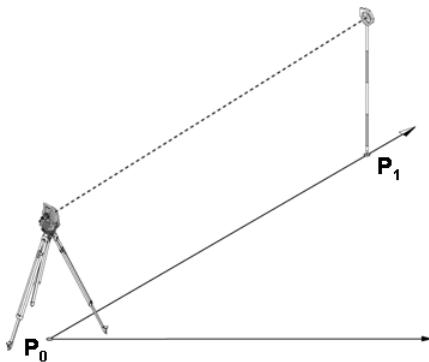
The position of the tool  $P_0$  and the orientation point  $P_1$  lie on a common building control line.
