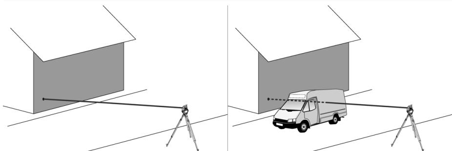
The laser beam is capable of measuring to any stationary target.
